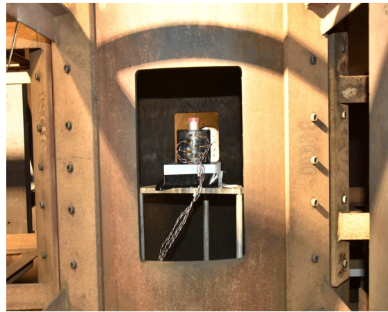
Collaboration between NPS and LLNL, and test setup for composite casing containing explosive material
