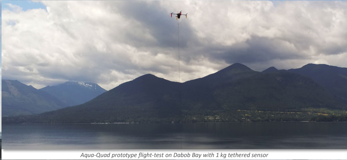
Aqua-Quad prototype flight-test on Dabob Bay with 1 kg tethered sensor
