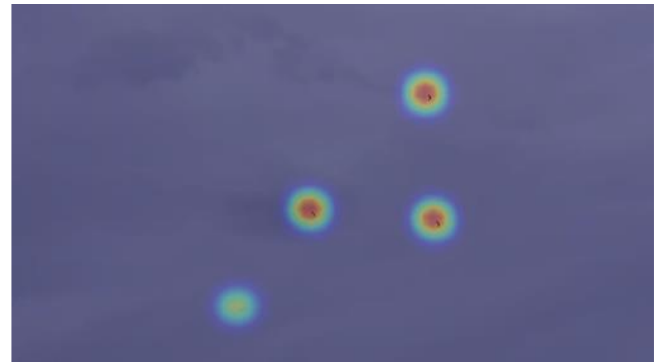
Detection of multiple identical UAS flying in formation during the integrated scenario.
