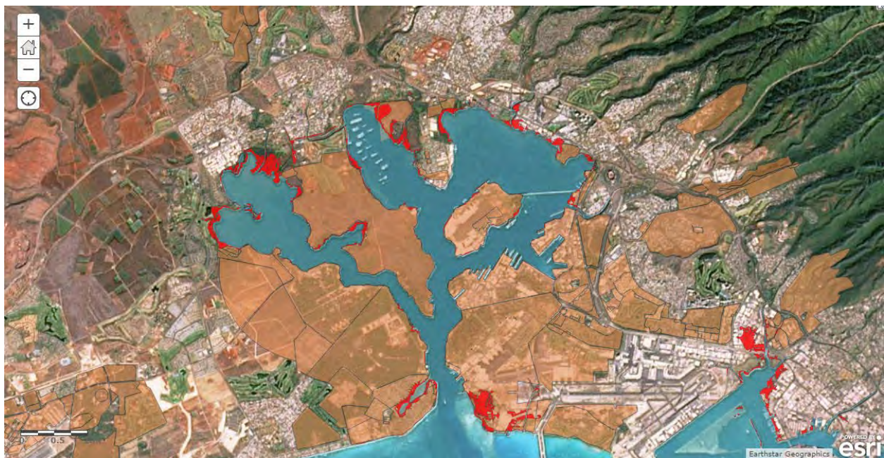
Figure 3. Example of use of spatial analysis to determine areas vulnerable to sea level rise. Here, DoD lands shown in brown are overlaid with the three-foot sea level rise flood model from NOAA, shown in red.
