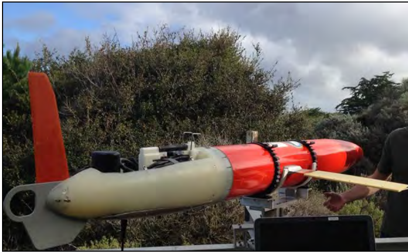
Figure 1. Modified NPS Spray glider with a mid-frequency Benthos DAT modem installed just forward of the tail (science bay cover is removed)
