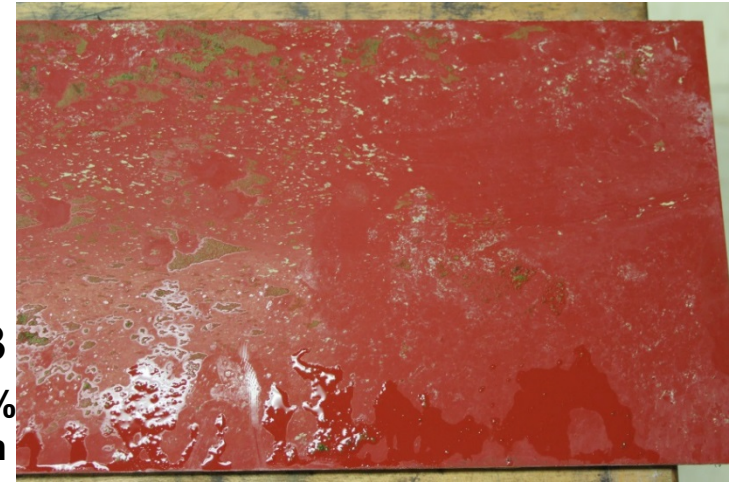
Specimen A coverage = 14.2% thickness, k = 520 \mu\text{m}
