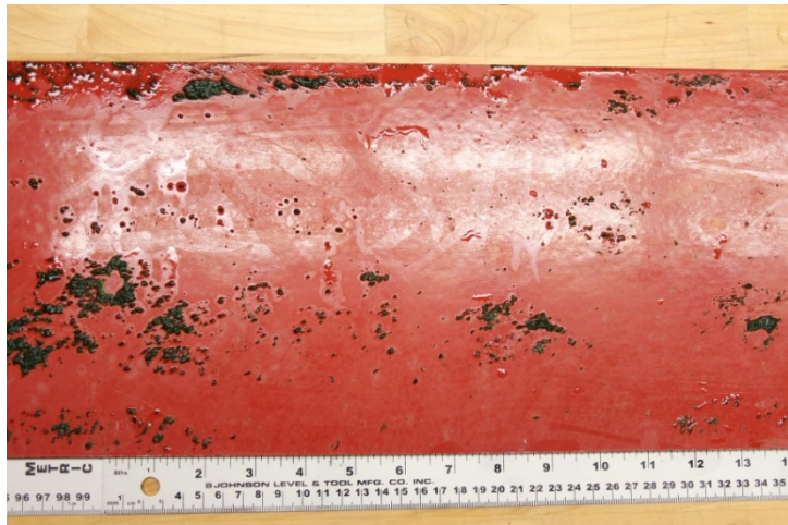
Specimen C coverage = 6.4% thickness, k = 574 \mu\text{m}
