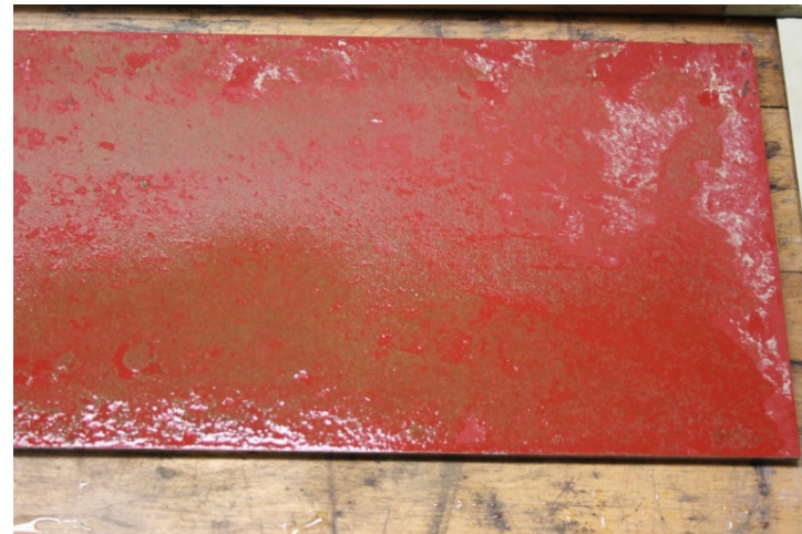
Specimen C coverage = 49.2% thickness, k = 98 \mu\text{m}
