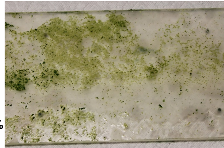
Specimen C coverage = 49.2% thickness, k = 98 \mu\text{m}
