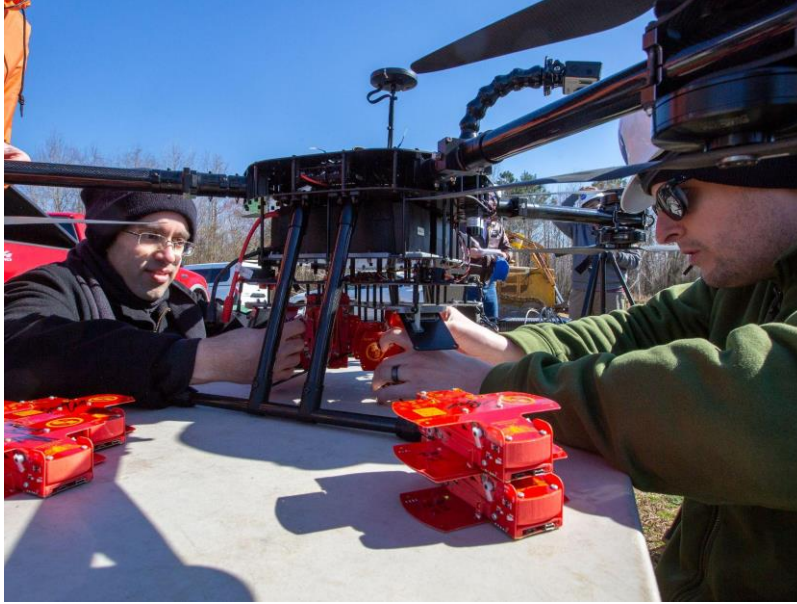
Figure 4: CICADA (Red Drones) and Deployment Drone 42
